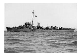
The USS England sank six Japanese submarines in just 12 days during May 1944. She bristled with anti-submarine weapons including two depth charge racks at the ship's stern, eight K-guns that shot depth charges out to 150 yards and a British designed, very deadly, 24 barrel Hedgehog anti-submarine mortar.
